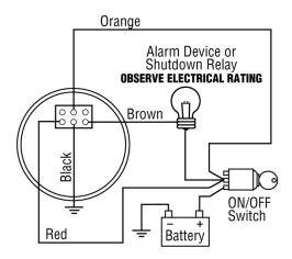
CAUTION: Devices containing solid state components can be damaged or caused to malfunction when used in systems which incorporate inductive loads (e.g. relays, solenoids, etc.) that can generate voltage spikes.
